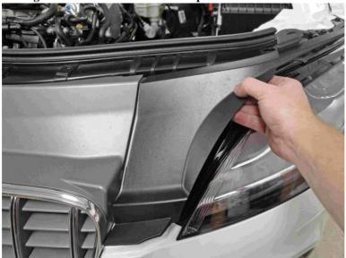
You can now remove the torx screws underneath each of these panels, as well as the screws located at the upper center portion of the grill next to the hood latch mechanism.
