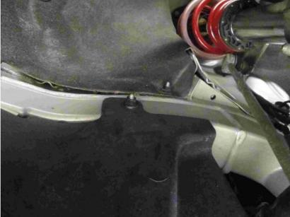
You will now need to pull back the fabric portion of the fender liner to expose the 2 nuts securing the bumper to the fenders. Remove these.
