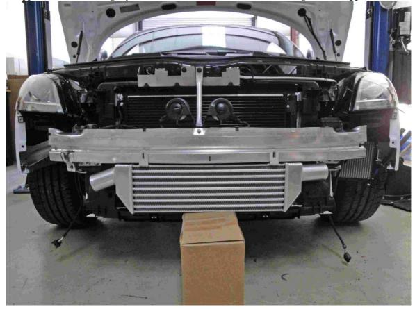
With the markings in place for the core mounting tabs, remove the core and use your power drill and 8.5mm drill bit to drill holes through the bumper support at these two markings. The support is hollow, so holes will need to be drilled through both the forward and rearward walls of the support. Please exercise caution to ensure that the drill bit does not extend so far out of the bit holder so as not to damage the AC condenser when the rear wall of the bumper support is punctured.
