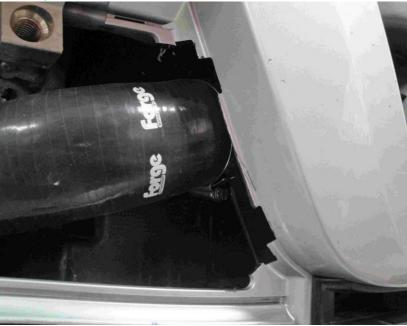
With the bumper itself now trimmed, you will now need to trim the passenger side (UK driver's side) grill backing panel to match the other side to allow for clearance for the hose. Obviously the driver's side panel has an opening to allow airflow to the secondary radiator, while the other side is blank, so the goal is to cut a matching hole into the blank panel.
