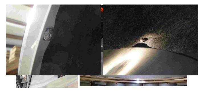
Remove all of the torx screws from the lower under tray in order to remove it. There are 19-21 screws total.
