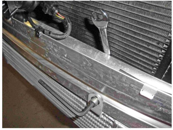
With the core now fitted, you will install the supplied silicone hoses to join together all of the intercooler and piping connections. The aluminium supports underneath the car, while obtrusive, should not prevent fitment of the hoses.
