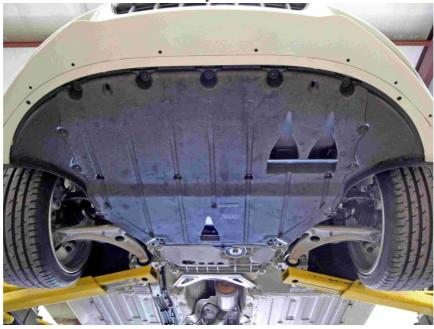
Now you will remove the corner pieces to the undertray which also extend upwards into the wheel wells as the lower part of the fender liners. There is a 10mm nut securing the back section to the frame and multiple torx screws securing them to the bumper. There are also 2 torx screws securing the fabric portion of the fender liner that need to be removed.
