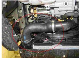
Remove the o-ring seal from the metal coupler end of the original intercooler hoses and fit them to the included corresponding new aluminium hose couplings as pictured below.
