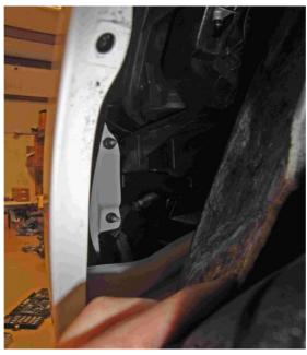
The bumper now needs to be slid forward to be lifted clear of the front end. Be sure to disconnect the wiring connectors to the fog lights. If your vehicle is equipped with headlight washers, you will also need to disconnect the washer fluid hose by releasing the small white clip and either plug the end of the hose or allow the fluid to drain into a container to be refilled later. This process is much easier with a friend assisting you.
