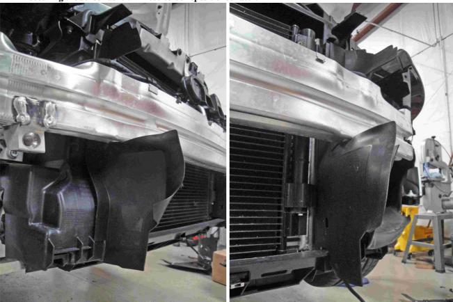
You will also need to remove the plastic air scoop for the secondary radiator to make room for the TWINtercooler hoses. If you so choose, you may modify this scoop yourself to retain some of it, however, removing it entirely is the easiest solution, and we have seen no problems from it. There are two round clips securing this piece to the secondary radiator that need to be released.
