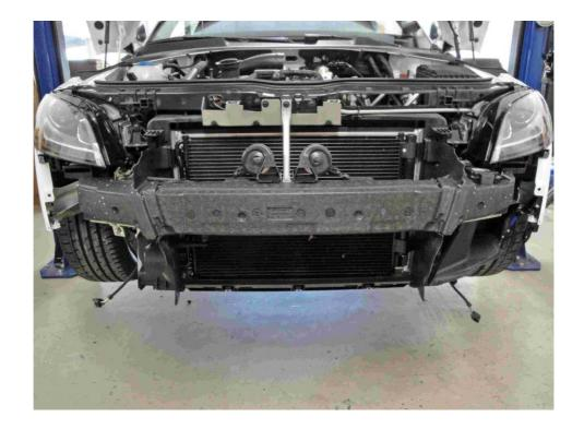
You will also remove both black plastic air guides and work them out from behind the bumper support. They have two plastic push in clips that need to be disconnected to remove them. This can be done with a flat blade screw driver. The external air temperature sensor is attached to one of these. Release the clip securing the sensor as it will need to be repositioned later.
